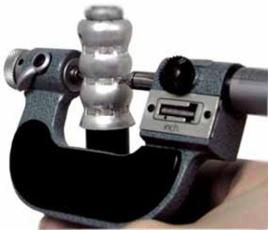
Figure 3 Measuring the crimp with a micrometer.
