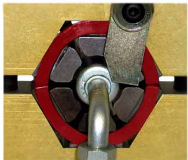
Figure 6 The proper method of using the locator flag.
