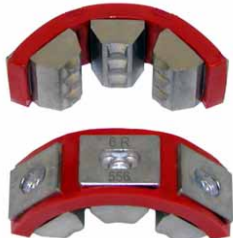
Figure 4 Identification of die sizes.
