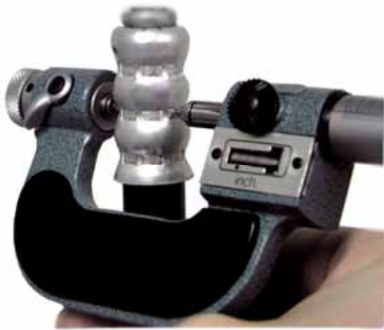
Figure 3 Measuring the crimp with a micrometer.
